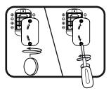
4. Replace the battery cover and tighten the screw to secure the battery cover.
